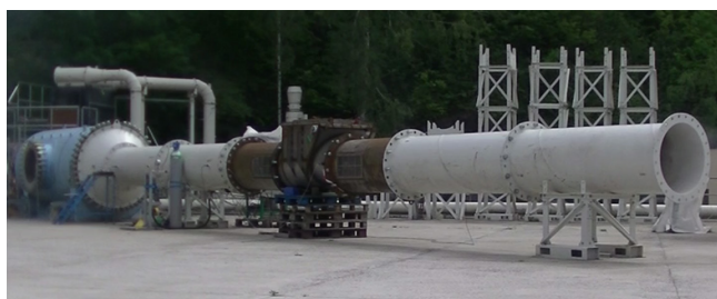
Flap valve test with INERIS notified body
